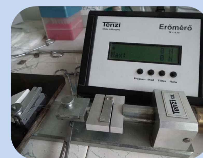
Pull-out Test (Tenzi)
